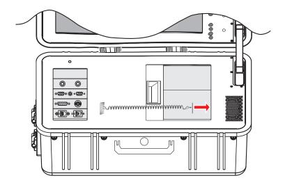
By sticking the remote tether to the inside wall of the accessory storage compartment:
